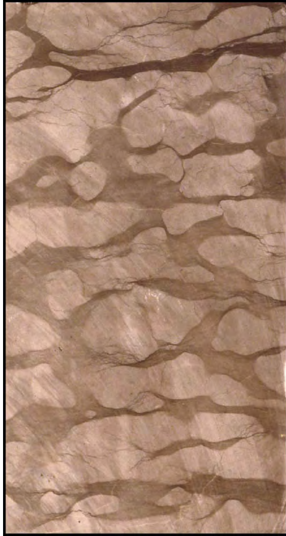
Figure 7. Slab photograph of nodular wackestone, Wink Formation. These wackestones contain scattered fragments of trilobites, thin-walled brachiopods, and ostracodes and locally grade into mudstone. Austral Oil Co., University No. 1, Andrews County, Texas. Depth: 12,030 ft. Slab is 8 cm wide.
