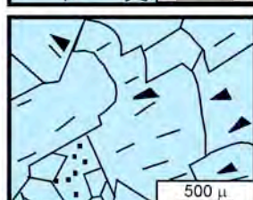
Figure 18. Dolomite textures described by Amthor and Friedman (1991). Figure from Amthor and Friedman (1991).
