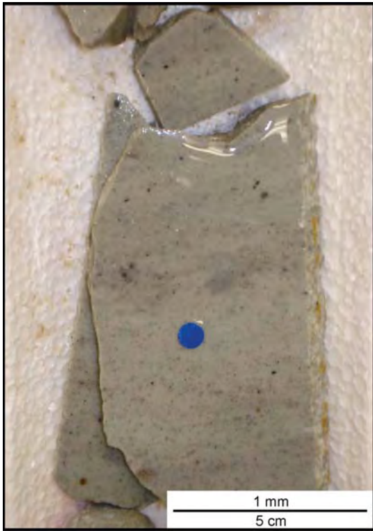
Figure 23. Core photo and thin section photomicrograph of crinoid wackestone, Dollarhide field 25-2-S, 8452 ft. Note crinoid fragment (pleochroic in polarized light) and a lack of porosity.
